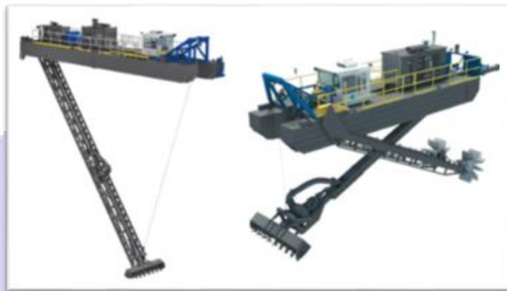
Versi-Dredge® (Sediment Removal)
